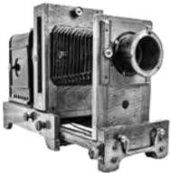
Taking a photograph involves allowing focused light to fall upon sensitised material, which is then processed to create an image. Initially, large glass plates were used in large wooden cameras like this. Although producing great images, but speed and portability were the main drawbacks.
